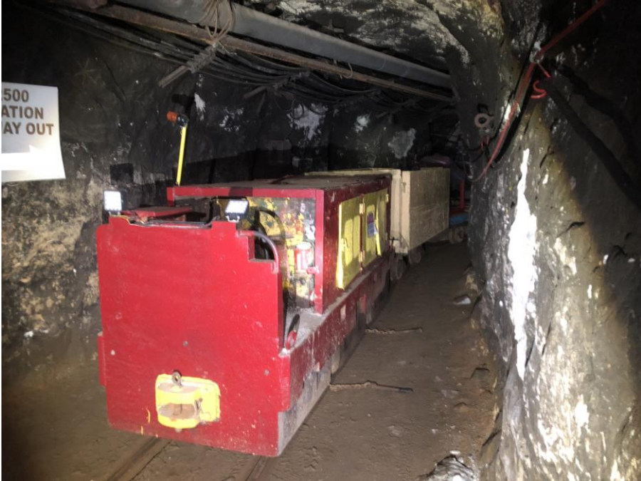
Figure 4 – Existing Locomotive and 8-Ton Rail Cars which Hauled 2,400 Tons per Day from the Historic #2 Mine
