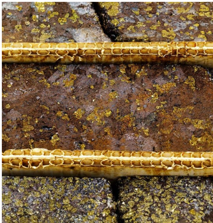
Figure 3 – Drill Core from Hole SX18-2441 Showing High-Grade, Coarse-Grained Sphalerite (Section of Two-Foot Interval Assaying 33% Zinc)
